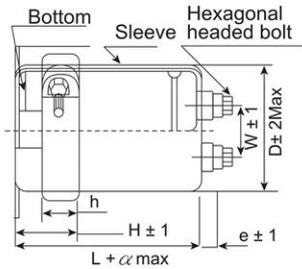
3-leg brackets for  $\phi 90$  capacitors have different hote shapes from the ordinary ones as illustrated below.
